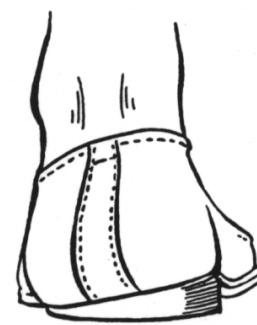
Fig. 8: Typical wear pattern of heel toplift on lateral-rear corner of heel, causing faulty tread and gait instability.
